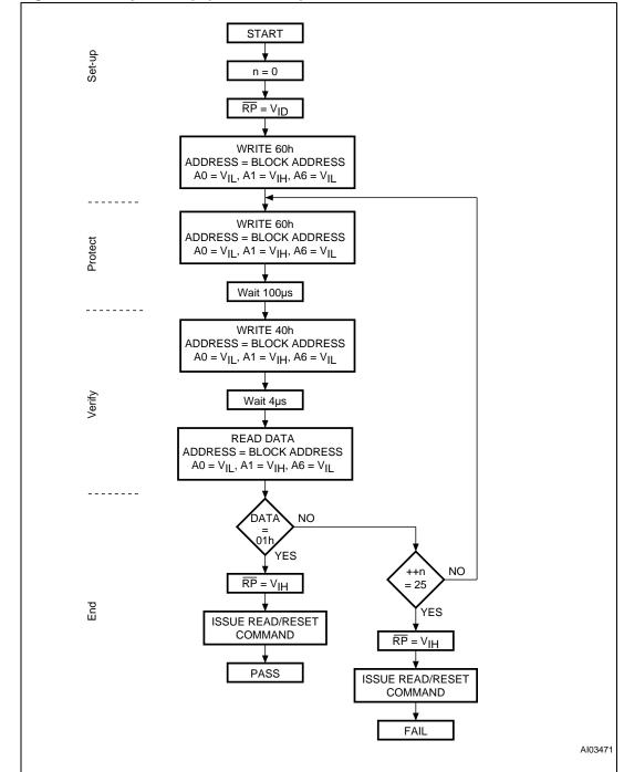
Figure 20. In-system equipment block protect flowchart
