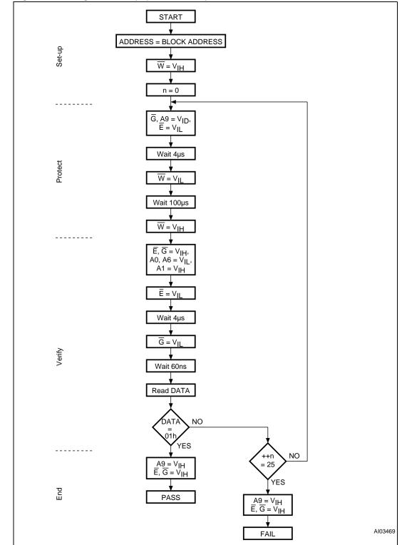
Figure 18. Programmer equipment block protect flowchart
