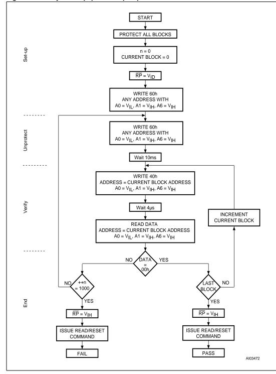
Figure 21. In-system equipment chip unprotect flowchart
