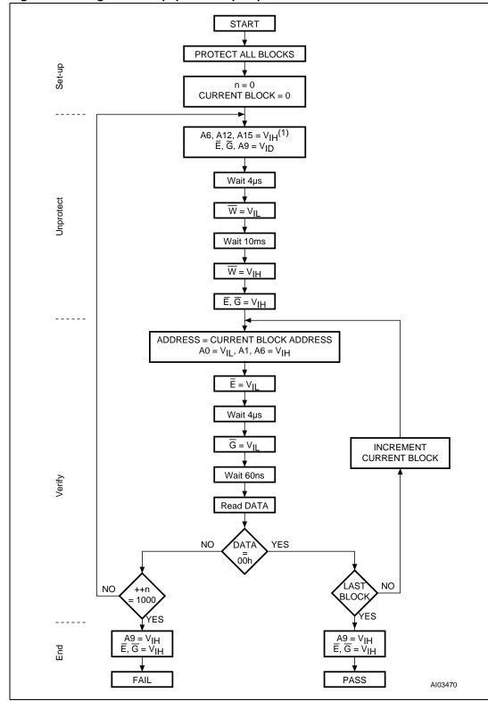
Figure 19. Programmer equipment chip unprotect flowchart
