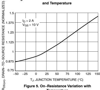
Figure 5. On-Resistance Variation with **Temperature**
