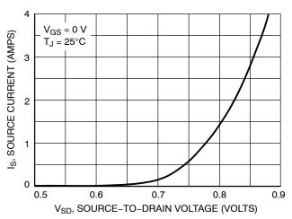
Figure 10. Diode Forward Voltage versus Current
