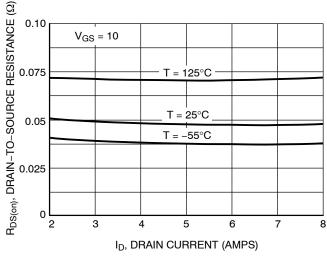
Figure 3. On-Resistance versus Drain Current
