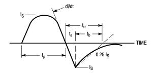
Figure 14. Diode Reverse Recovery Waveform
