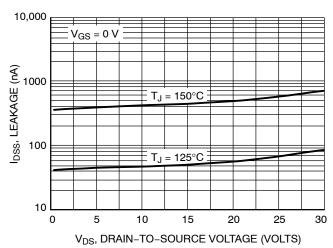
Figure 6. Drain-to-Source Leakage Current versus Voltage
