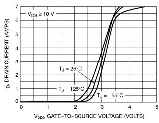
Figure 2. Transfer Characteristics
