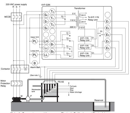
Note: 1. Be sure to ground the common Electrode E<sub>5</sub> (the longest Electrode).
