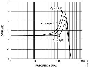
Figure 13. Small Signal Frequency Response for Various  $C_L$ ,  $V_{OUT} = 500 \text{ mV } p\text{-}p$ ,  $V_S = 5 \text{ V}$ , G = +1
