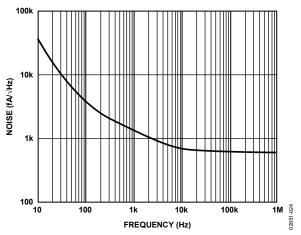
Figure 24. Input Current Noise vs. Frequency
