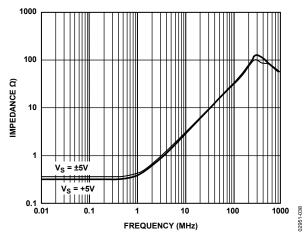
Figure 38. Output Impedance vs. Frequency
