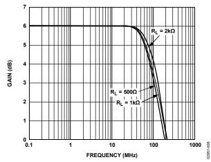
Figure 8. Small Signal Frequency Response for Various R<sub>L</sub>,  $V_S = \pm 5 V$ ,  $V_{OUT} = 500 \text{ mV } p$ -p
