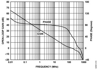
Figure 15. Open-Loop Gain and Phase,  $V_S = \pm 5 V$
