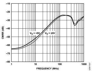
Figure 37. CMRR vs. Frequency,  $V_{IN} = 1 V p-p$
