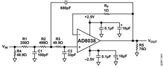
Figure 44. Low-Pass Filter for Video
