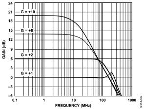
Figure 4. Small Signal Frequency Response for Various Gains,  $V_{OUT} = 500 \text{ mV } p\text{-}p$ ,  $V_S = \pm 5 \text{ V}$
