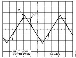
Figure 34. Output Overdrive Recovery, Gain = +2
