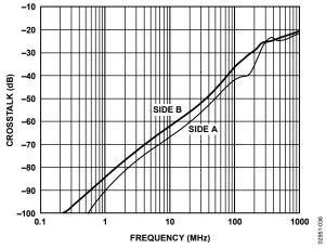
Figure 36. AD8039 Crosstalk,  $V_{IN} = 1 \text{ V p-p, Gain} = +1$
