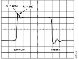
Figure 25. Small Signal Transient Response for Various  $R_L$ ,  $V_S = 5 V$
