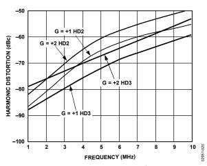
Figure 20. Harmonic Distortion vs. Frequency for Various Gains,  $V_s = 5 V$ ,  $V_{OUT} = 2 V p - p$
