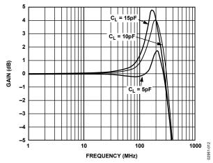
Figure 12. Small Signal Frequency Response for Various  $C_{L_r}$  $V_{OUT} = 500 \text{ mV } p\text{-}p$ ,  $V_S = \pm 5 \text{ V}$ , G = +1
