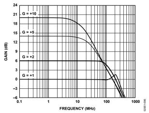
Figure 6. Small Signal Frequency Response for Various Gains,  $V_{OUT} = 500 \text{ mV } p\text{-}p$
