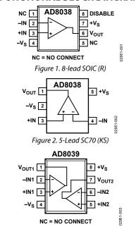
Figure 3. 8-Lead SOIC (R) and 8-Lead SOT-23 (RJ)
