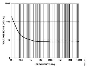
Figure 23. Input Voltage Noise vs. Frequency
