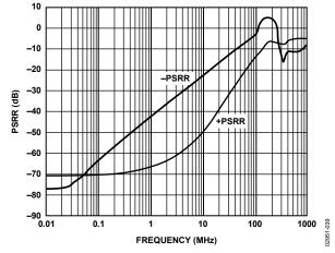
Figure 39. PSRR vs. Frequency
