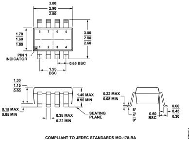
Figure 48. 8-Lead Small Outline Transistor Package [SOT-23] (RJ-8) Dimensions shown in millimeters
