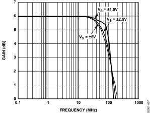
Figure 7. Small Signal Frequency Response for Various Supplies,  $V_{OUT} = 500 \text{ mV } p\text{-}p$
