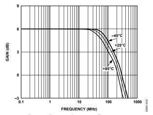
Figure 16. Frequency Response vs. Temperature, Gain = +2,  $V_S = \pm 5 V$ ,  $V_{OUT} = 2 V p-p$
