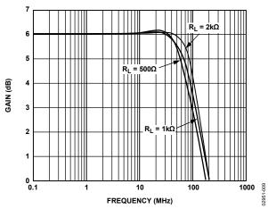
Figure 9. Small Signal Frequency Response for Various  $R_L$ ,  $V_S = 5 V$ ,  $V_{OUT} = 500 \text{ mV } p\text{-}p$
