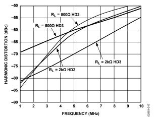
Figure 17. Harmonic Distortion vs. Frequency for Various Loads,  $V_S = \pm 5 V$ ,  $V_{OUT} = 2 V p$ -p, G = +2
