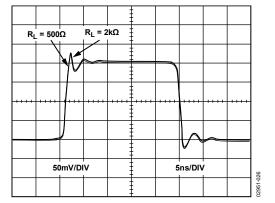
Figure 26. Small Signal Transient Response for Various  $R_L$ ,  $V_S = \pm 5 V$
