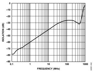
Figure 42. AD8038 Input-Output Isolation (G = +2,  $R_L = 2 k\Omega$ ,  $V_S = \pm 5 V$ )
