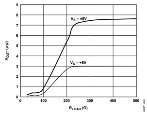
Figure 40. Output Swing vs. Load Resistance
