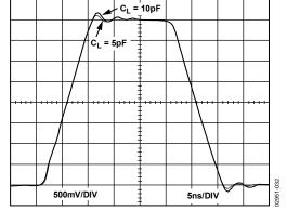
Figure 32. Large Signal Transient Response for Various  $C_L$ ,  $V_S = \pm 5 V$
