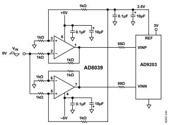
Figure 43. Schematic to Drive AD9203 with the AD8039
