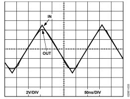
Figure 33. Input Overdrive Recovery, Gain = +1
