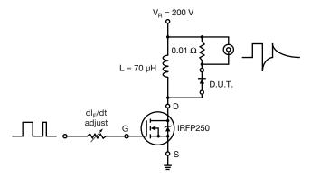
Fig. 10 - Reverse Recovery Parameter Test Circuit
