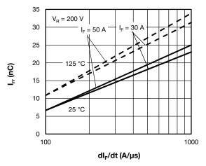
Fig. 9 - Typical Reverse Recovery Current vs. dl<sub>F</sub>/dt
