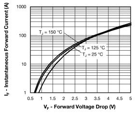
Fig. 1 - Typical Forward Voltage Drop Characteristics (Per Leg)
