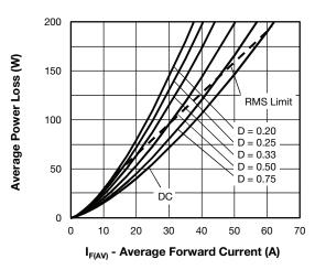
Fig. 6 - Forward Power Losses Characteristics (Per Leg)
