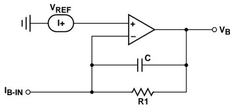
$$V_{REF} = 1.4 \text{ V} \pm 0.2 \text{ V(DC)}$$
