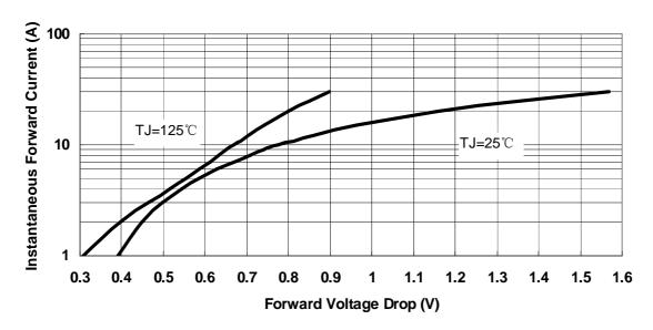
Fig.3-Typical Instantaneous Forward Voltage Characteristics
