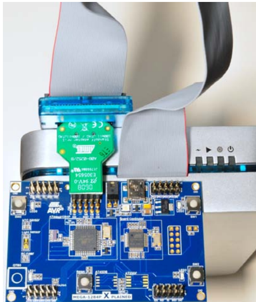
Figure 4-3. Connecting AVR ONE! to a Xplained board.
