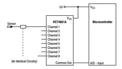
Figure 8. MC74HCT4851A Solution Solution by applying the HCT4851A multiplexer
