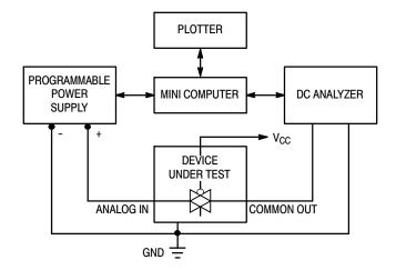
Figure 9. On Resistance Test Set-Up
