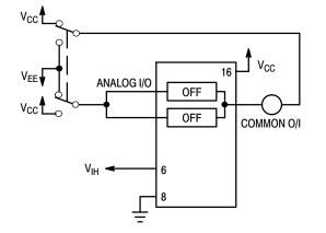
Figure 11. Maximum Off Channel Leakage Current, Common Channel, Test Set–Up
