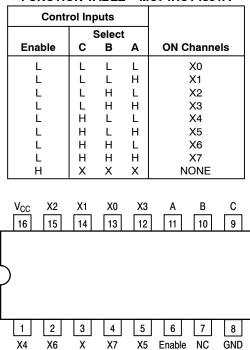
Figure 2. MC74HCT4851A 16-Lead Pinout (Top View)
