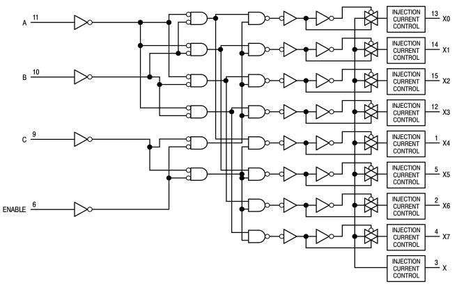
Figure 21. Function Diagram, HCT4851A
