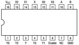
Figure 4. MC74HCT4852A 16-Lead Pinout (Top View)
