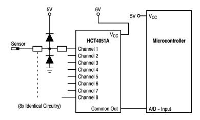
Figure 7. Actual Technology Requires 32 passive components and one extra 6V regulator to suppress injection current into a standard HCT4051 multiplexer
