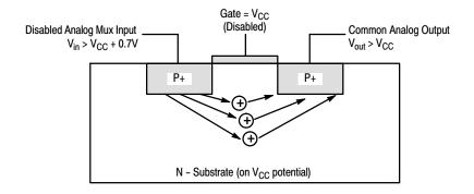
Figure 20. Diagram of Bipolar Coupling Mechanism
