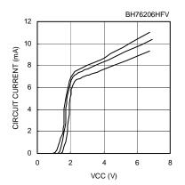
Fig.15 Supply Voltage-Circuit Curren
