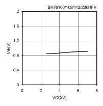
Fig.27 Supply Voltage-Vth
