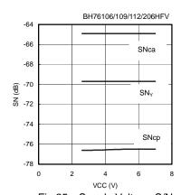
Fig.25 Supply Voltage-S/N
