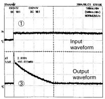
Fig10 Relationship of Output Voltage to Input Voltage (For BH76106HFV Cin=1uF)
