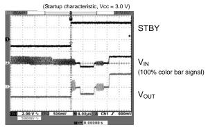
Fig.5 Standby Response Characteristic
