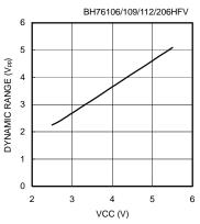
Fig.19 Dynamic Range Characteristic (VCC Characteristic)
