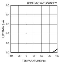
Fig.16 Temperature-Standby Circuit Current
