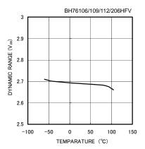
Fig.20 Dynamic Range Characteristic (Temperature Characteristic)
