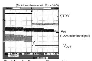
Fig.6 Standby Response Characteristic
