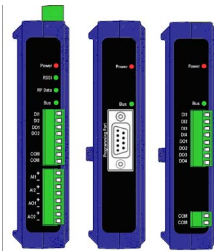
Figure 7 Front View of Zlinx Wireless I/O Base, Configuration Box, and Expansion Modules,
