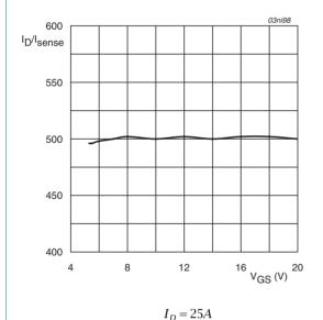
Fig 15. Drain-sense current ratio as a function of gate-source voltage; typical values
