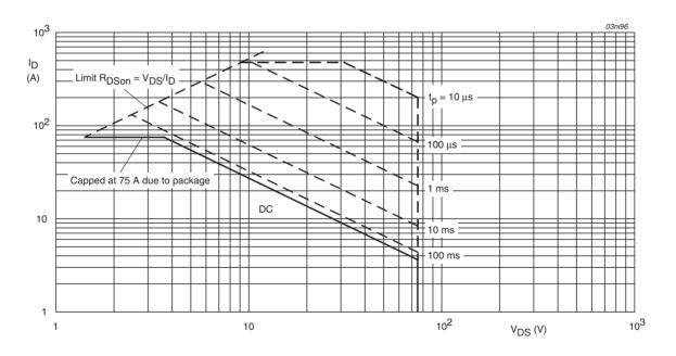
$T_{mb} = 25$ °C; $I_{DM}$ is single pulse
