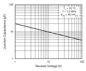
Fig. 5 - Typical Junction Capacitance
