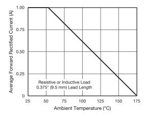
Fig. 1 - Forward Current Derating Curve
