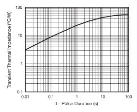
Fig. 6 - Typical Transient Thermal Impedance
