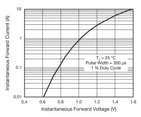
Fig. 3 - Typical Instantaneous Forward Characteristics
