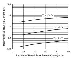
Fig. 4 - Typical Reverse Characteristics
