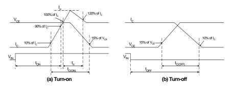
Fig. 4. Switching Time Definition
