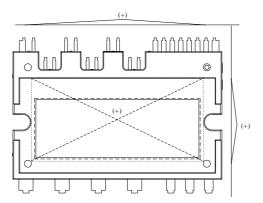
Fig. 5. Flatness Measurement Position
