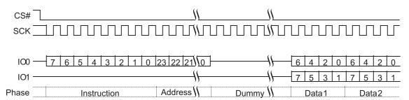
Figure 3.8 Quad Output Command without Latency
