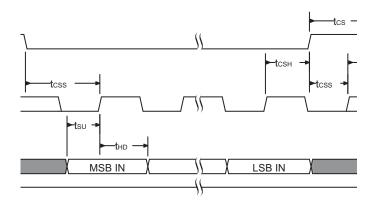
Figure 4.9 SPI Single Bit Output Timing
