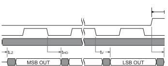
Figure 4.10 SPI MIO Timing
