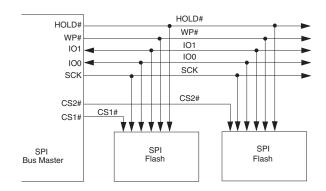
Figure 2.4 Bus Master and Memory Devices on the SPI Bus – Quad Bit Data Path
