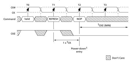
Note: 1. The earliest precharge power-down entry may occur is at T2, which is 1 × <sup>t</sup>CK after the REFRESH command. Precharge power-down entry occurs prior to <sup>t</sup>RFC (MIN) being satisfied.
