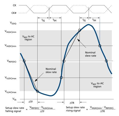
Figure 24: Tangent Line for <sup>t</sup>IS
