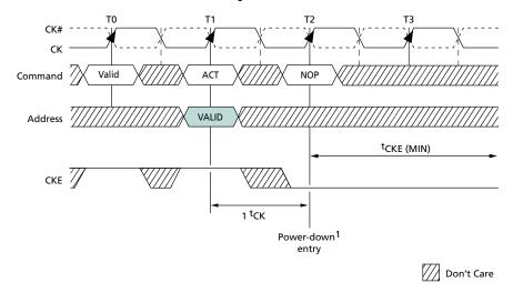
Note: 1. The earliest active power-down entry may occur is at T2, which is 1 × <sup>t</sup>CK after the ACTI-VATE command. Active power-down entry occurs prior to <sup>t</sup>RCD (MIN) being satisfied.
