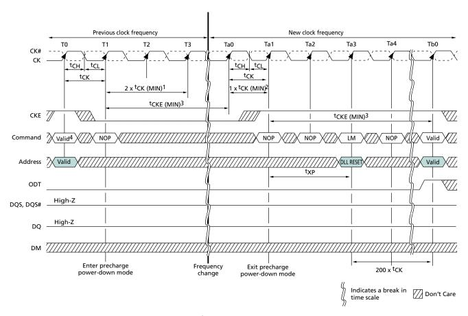
Notes: 1. A minimum of 2 × <sup>t</sup>CK is required after entering precharge power-down prior to changing clock frequencies.
