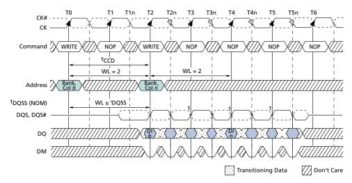
1. Subsequent rising DQS signals must align to the clock within <sup>t</sup>DQSS.
