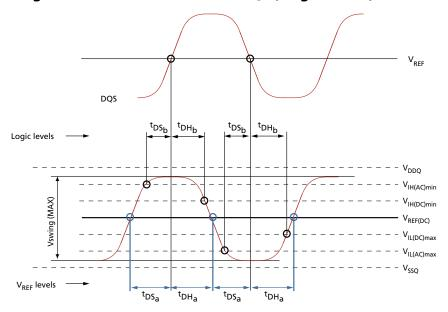
Figure 34: AC Input Test Signal Waveform (Differential)
