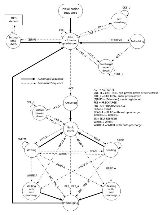
Note: 1. This diagram provides the basic command flow. It is not comprehensive and does not identify all timing requirements or possible command restrictions such as multibank interaction, power down, entry/exit, etc.
