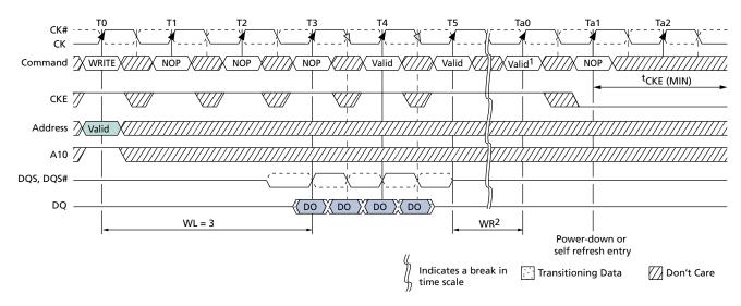
Notes: 1. Internal PRECHARGE occurs at Ta0 when WR has completed; power-down entry may occur 1 x <sup>t</sup>CK later at Ta1, prior to <sup>t</sup>RP being satisfied.
