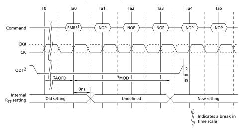
Notes: 1. The LM command is directed to the mode register, which updates the information in EMR (A6, A2), that is,  $R_{TT}$  (nominal).
