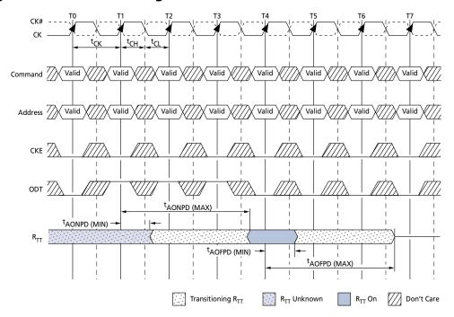
Figure 84: ODT Turn-Off Timings When Entering Power-Down Mode
