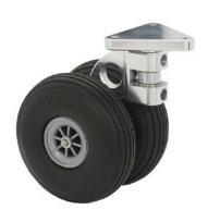
This kit contains a single, precision-machined caster assembly (two are required if you're mounting them to our Arlo Robot Base Kit - #28960). High-quality 6061 machined aluminum components (created in our machine shop in Rocklin, CA), are combined with smooth-rolling ball bearings and durable 3-inch Du-Bro pneumatic rubber tires. The dual independent tire design reduces vibration and drag, as well as increasing its load-carrying capacity.
