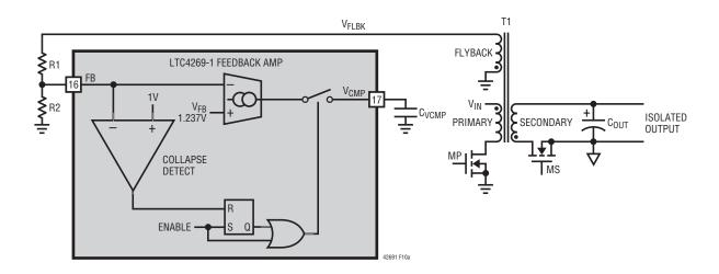
Figure 10a. LTC4269-1 Switching Regulator Feedback Amplifier
