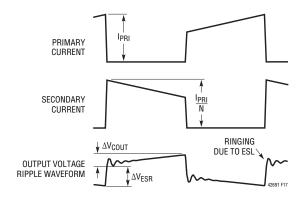
Figure 17. Typical Flyback Converter Waveforms
