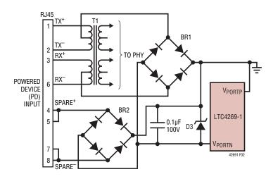
Figure 2. PD Front End Using Diode Bridges on Main and Spare Inputs
