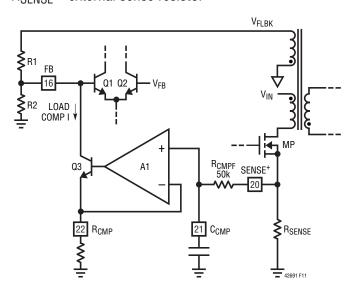
Figure 11. Load Compensation Diagram
