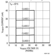
Input Current vs Input Voltage
