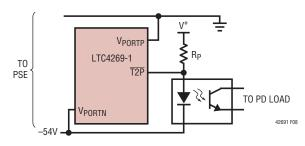
OPTION 2: SHUNT CONFIGURATION FOR ACTIVE HIGH/OPEN COLLECTOR OUTPUT
