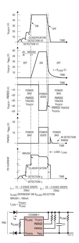
Figure 1. V<sub>NEG</sub>, PWRGD, PWRGD and PD Current as a Function of Input Voltage
