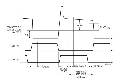
Figure 10b. LTC4269-1 Switching Regulator Timing Diagram
