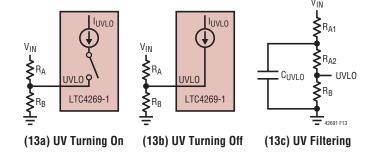
Figure 13. UVLO Pin Function and Recommended Filtering
