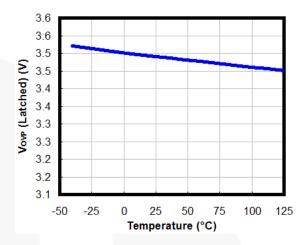
Figure 54. Non-Latching OVP vs. Temperature
