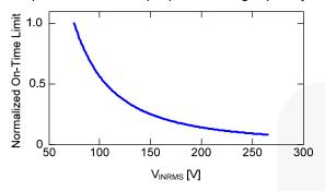
Figure 14. On-Time vs. V<sub>IN\_RMS</sub>
