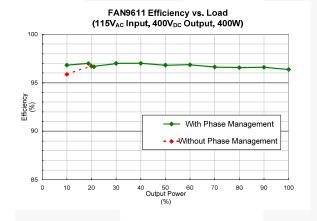
Figure 62. Measured Efficiency at 115V<sub>AC</sub> (Default Thresholds)
