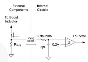
Figure 26. Current-Sense Protection Circuits
