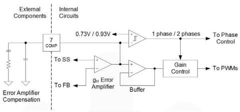
Figure 20. Error Amplifier Compensation Circuitry
