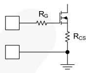
Figure 33. Recommended Gate Drive Schematic
