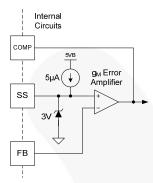
Figure 27. FAN9611 Error Amplifier Configuration
