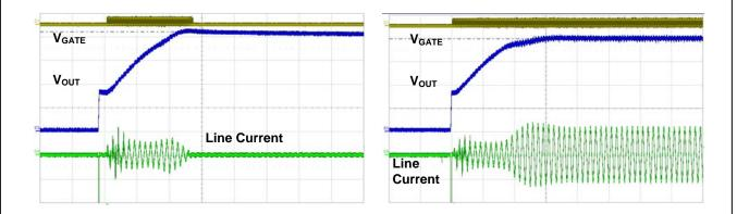
Figure 59. No-Load Startup at 115 V<sub>AC</sub>
