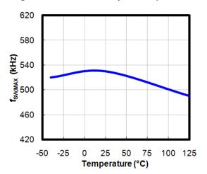
Figure 51. Restart Timer Frequency vs. Temperature
