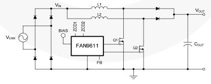
Figure 1. Simplified Application Diagram
