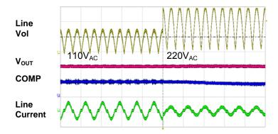
Figure 61. Input Voltage Feedforward
