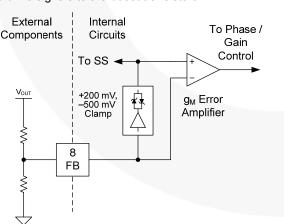
Figure 21. Output-Voltage Feedback Circuit
