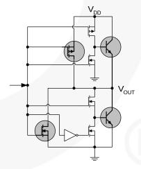
Figure 25. Current-Sense Protection Circuits
