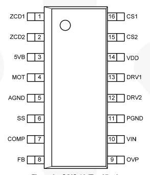
Figure 2. SOIC-16 (Top View)
