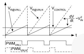
Figure 10. Input-Voltage Feedforward
