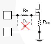
Figure 34. Discharge Diode is Not Recommended
