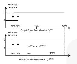
Figure 28. Adjusting Phase Management Thresholds
