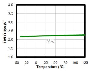
Figure 38. UVLO Thresholds vs. Temperature
