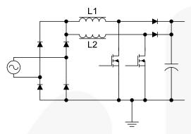
Figure 8. Interleaved PFC Boost Operation
