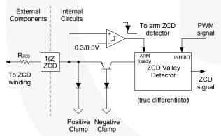
Figure 16. Zero-Current Detect Circuit
