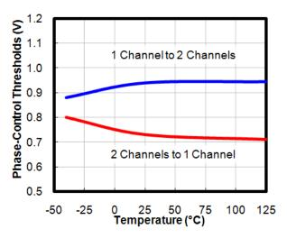
Figure 46. Phase-Control Thresholds vs. Temperature
