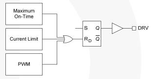
Figure 13. Conduction Interval Termination
