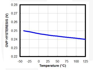
Figure 56. OVP Hysteresis vs. Temperature
