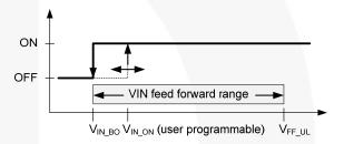
Figure 30. VIN Turn-on and Turn-off Thresholds
