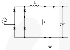
Figure 6. Basic PFC Boost Converter
