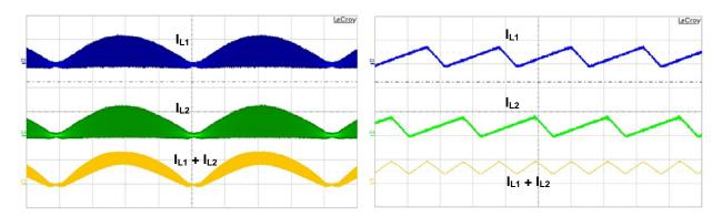
Figure 57. Ripple-Current Cancellation (110 V<sub>AC</sub>)
