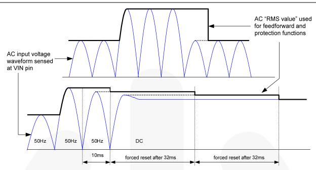
Figure 24. Input Voltage Sensing Waveforms
