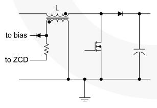
Figure 11. Simple Zero-Current Detection Method
