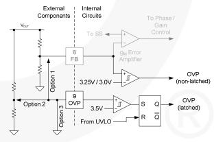
Figure 22. Secondary Over-Voltage Protection Circuit
