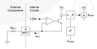
Figure 18. Maximum On-Time Control (MOT)
