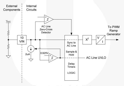
Figure 23. Input Voltage Sensing Circuit
