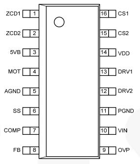
Figure 5. Pin Layout (Top-View)
