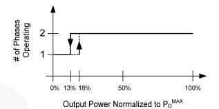
Figure 15. Automatic Phase-Control Operation
