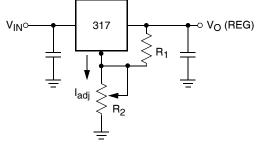
$V_O (REG) = 1.25V (1+R_2/R_1)+I_{adj} R_2$
