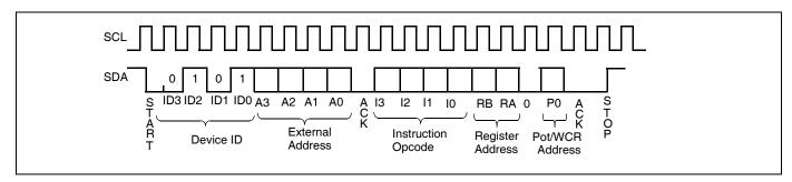
Figure 4. Three-Byte Instruction Sequence
