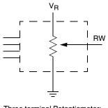
Three terminal Potentiometer; Variable voltage divider
