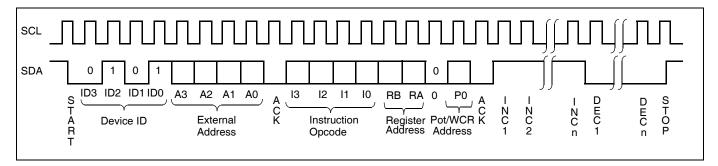
Figure 6. Increment/Decrement Timing Limits
