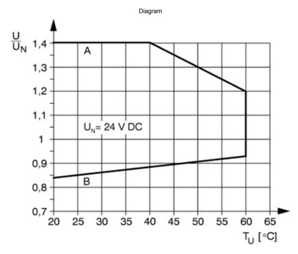
Curve A Maximum permissible continuous voltage  $U_{max}$  with limiting continuous current on the contact side (see relevant technical data) Curve B Minimum permissible operate voltage  $U_{op}$  after pre-excitation (see relevant technical data)
